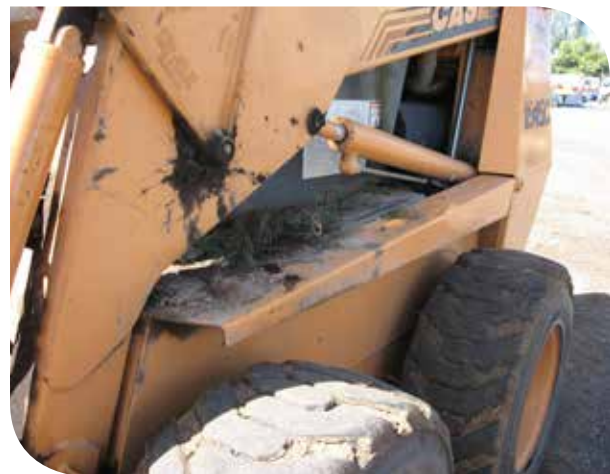
Plant material attached to bobcat.
